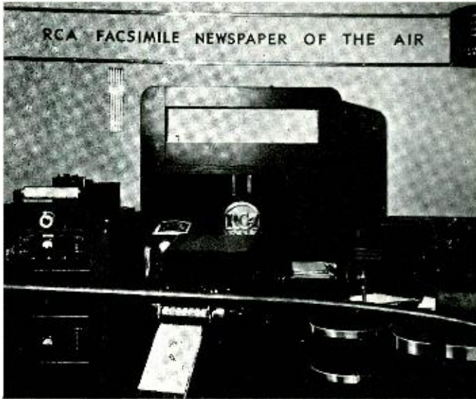
Fig. 4—A section of the facsimile exhibit showing scanner, “horizontal” receiver, and home receiver in operation.
